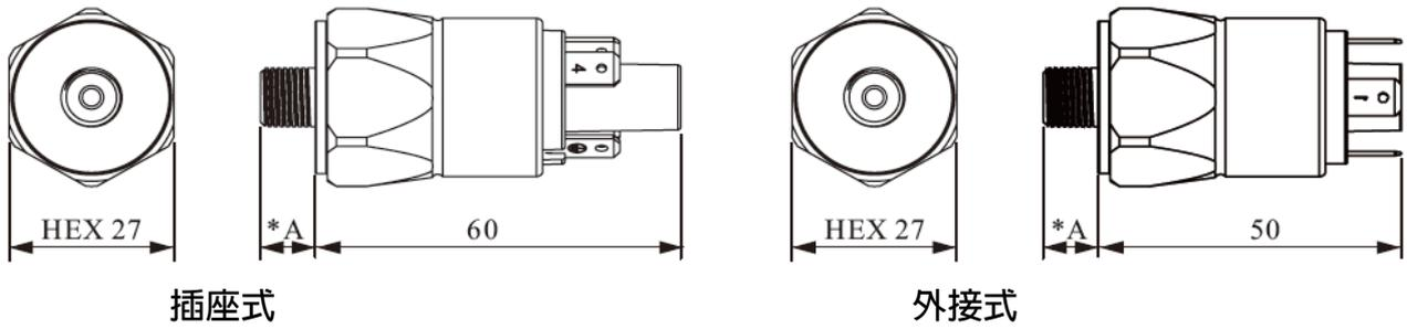
\*A: 9mm - M10 x 1 (taper), M10 x 1, G1/8" , 1/8" PT, 1/8" NPT      \*A: 12mm - M12 x 1.5, G1/4" , 1/4" PT, 1/4" NPT
